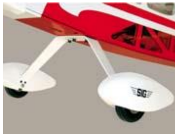
Factory painted aluminum main landing gear with fiberglass wheel pants.
