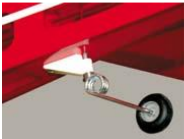
Features a strong steerable tailwheel assembly.
